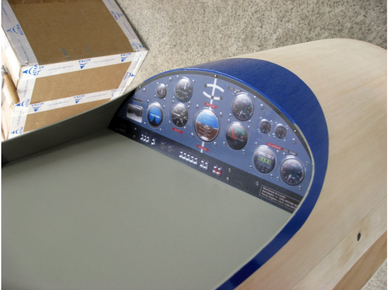
The interior of the cabin is coated, everything is prepared for the final sealing of the molding of the cabin.
