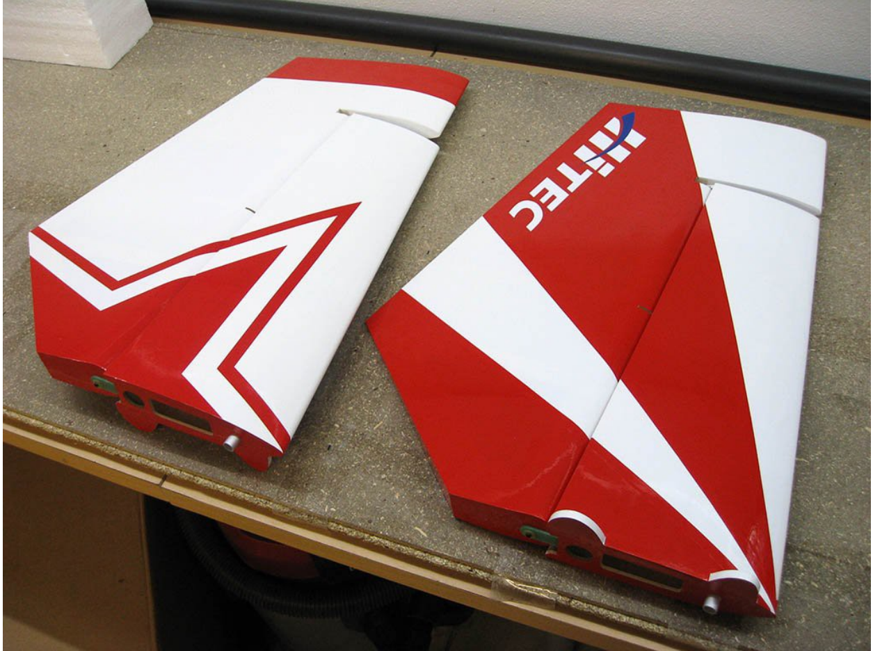
Sticker and star is cut on CNC plotter from car foil.
