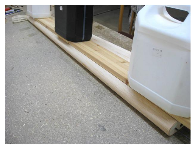
Once the cover is fully bent, it is loaded with a flat board to ensure that the cover is flush against all ribs. The bonding to the structure is carried out only after the pre-bent coating has completely dried.
