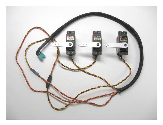
After powering, the smaller tubing shrinks first and the cables are angled as needed. The braid is then set up and shrinked together with the power and shrink cables. The result is neat and quite durable. After mounting into the structure, the servos must be programmed sequentially, first the two servos are synchronized and then the third one is added.
