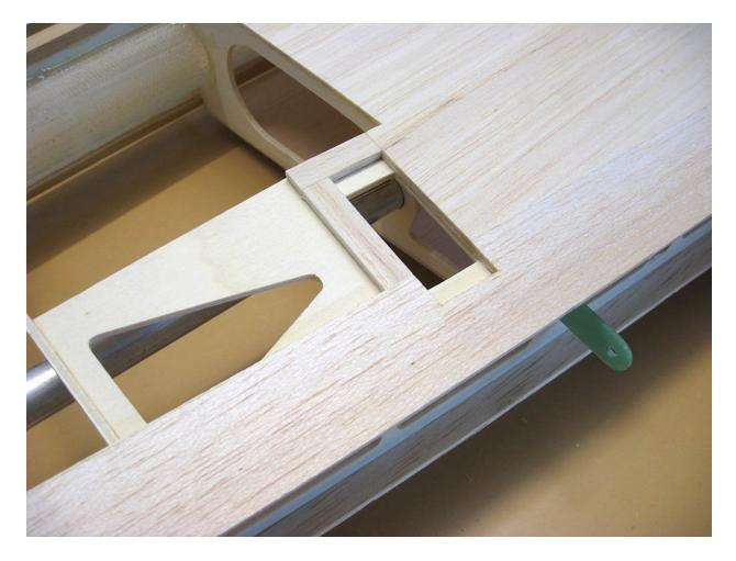
The first layer of 1.5 mm strips is made like other servos, the next layer is made directly by covering the root of the wing behind its main web.
