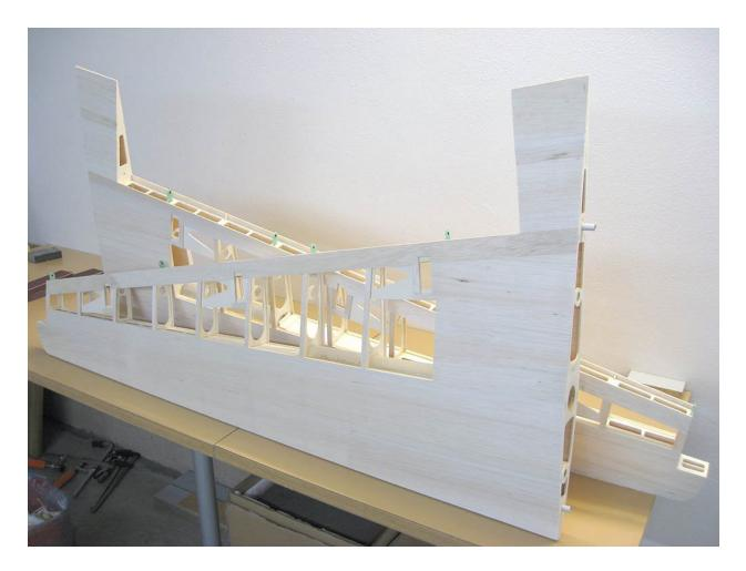
The wings are now banded and the overlapping covers have been trimmed and ground. To finish the construction of the wing, just stick the leading edges and end arches of thick balsa board.
