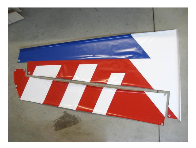
Ironing has been described elsewhere. Cutting parts of the cover and ironing the covers in the photo is for more than 2 hours of time. When cutting individual parts of the cover it is necessary to be accurate, otherwise in more complicated designs they will not be reasonably ironable;
