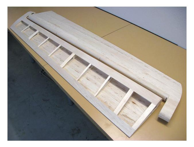
The wings of the ailerons are belted after counterweighting. A 20 mm band is glued to the root rib and to the ribs where the levers will be. The remaining ribs are striped with 10 mm wide strips. In version 2, thanks to the counterweights, the wings are really large.
