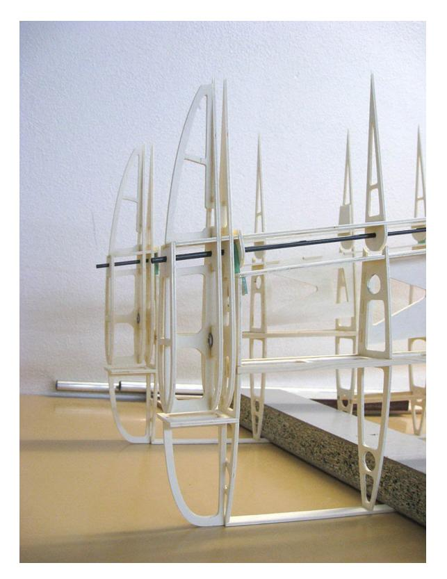
New wing arch design complete. On this construction, balsa will be glued to the side and the final shape of the arch will be shaped. The front part of the arch is not yet glued, the cover must be glued on the tubes, the tube must go into the ribs with the necessary overlap
