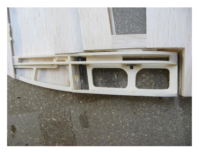
The SFG shaft must be lined with stronger balsa on the counterweight and runner. Before that, it is a good idea to glue one SFG and lining it so that the SFG snaps into place. The SFG is threaded through a carbon tube and an M4 flat head screw from the inside of the counterweight. Only now can the counterweight be coated. In the place of the leading edge it is coated with one piece of balsa, the plate must be soaked in advance and allowed to dry on the structure before gluing.
