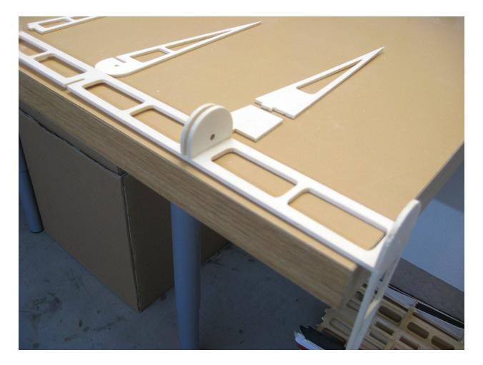
These parts must be glued really perpendicularly, otherwise the aileron will not walk freely in the curtains. It is good to try to insert a loose hinge between the two parts so check the gap, it should be slightly larger than 2 mm, which is the hinge thickness. It is good to wait for the adhesive to dry completely before continuing.
