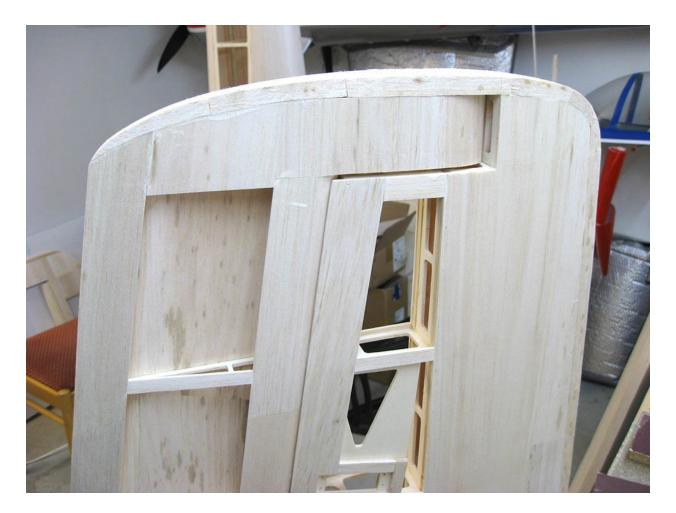
The aileron is fixed in the neutral position and the end arch blocks are glued. I glued from five pieces of board thickness. 12 mm. The photo shows the condition after trimming to the wing profile and after trimming to the final wing plan. The arc is then rounded before the arc is cut at the leading edge of the counterweight.
