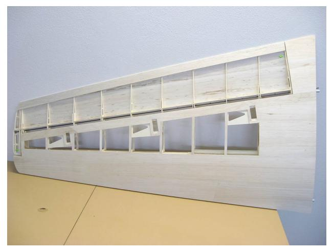
The aileron is trimmed together with the wing at the trailing edge and to the level of the counterweight structure. Subsequently, the wing joint cover is glued, the counterweight cover is glued and the ribs are finally banded. The wing is still missing the leading edge.
