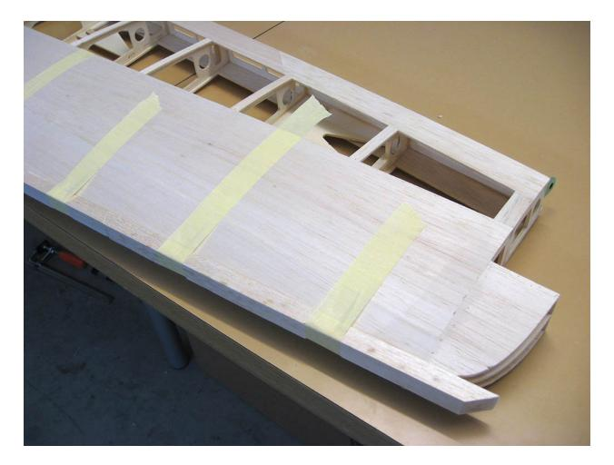
There is not much to explain here, the log must be extended to the required length, it is cut from a board of 12 mm thickness, on one side it has a width of 18 and on the other 15 mm. The tape is tightened, glued with a dispersion, preferably so that the adhesive does not flow, then it is severely cut and sanded.
