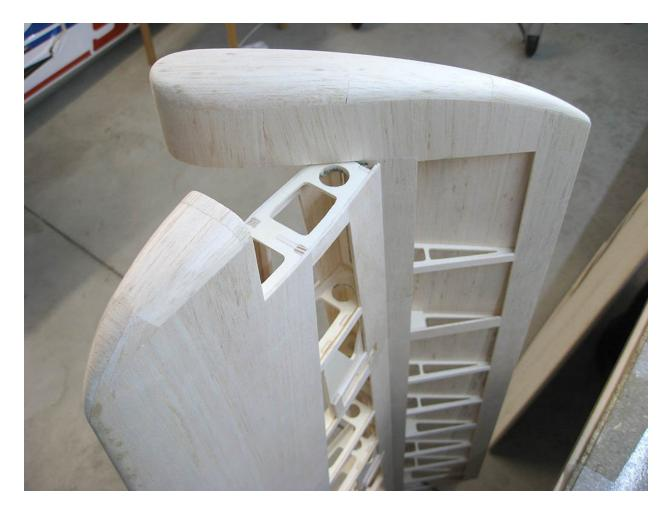
The counterweight is wider than a real aircraft to be more efficient and to help servos. Only after the flight will it be clear what the purpose of the counterweight is.
