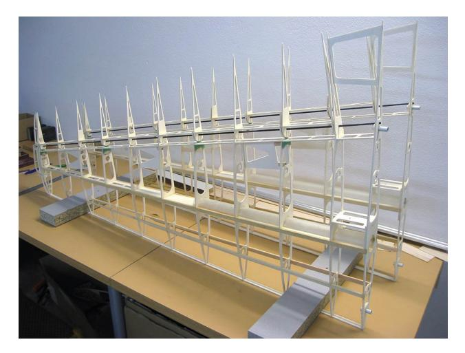
One motivational photo, the wings are ready to be coated, the basic construction is finished. The wing is in place. Maximum satisfaction, the aileron already walks freely, has no play and a deviation of +/- 60 degrees is smooth. The original version was a considerable problem, slits and curtains had to be grinded and there was a clearance, which with the operation even increased ...
