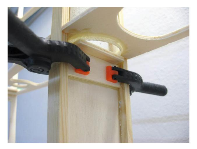
For the prototype, I managed to get a carbon tube that is slightly shorter than the original plan. I shortened the case with a one-sided plate of metal saws according to the mark I made when splicing with the fuselage. One piece of poplar plywood partially closes the sleeve, it must not close completely, it would then be very difficult to insert the pipe due to compressed air. The other two pieces of hollyhock close the opening in the web after the sleeve is shortened. It is glued with epoxy.
