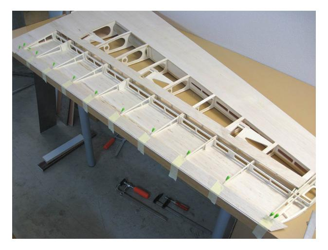
Drain board is width 33 mm from stronger balsa thickness. 2 mm, the board must be adjusted to the required length. The aileron remains on the wing and the whole is grounded so that the top cover of the aileron touches the entire surface of the table and the end of the aileron is flush with the edge of the table. The dispersion is then applied and the cutting board is first attached to the ribs on one side and the other side is pulled to the table with tape.
