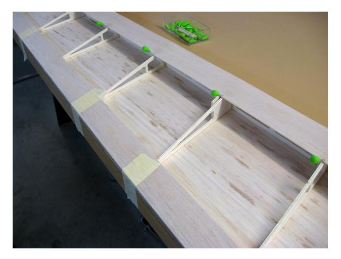
At the trailing edge, the aileron is glued with tape to a flat table, the aileron is loaded to fully rest on the table in all places. After applying sufficient amount of glue, the coating is gradually pinned to all ribs or even to the web.
