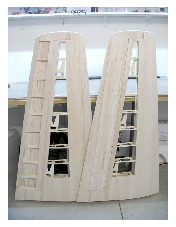
The wing with aileron should always have the same gap between each other in the ground plan, which should be about 2.5 mm in front of the coating film, if not, such gaps must be made. This is followed by the last preparation before film coating, sealing and fine sanding. In case of careful work, only small things are necessary to seal, fine sanding only removes balsa hairs and generally smooths the construction surface so that it does not protrude into the foil coating for years.
