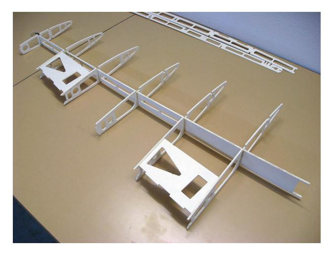
The rows are first glued ribs and before they completely dry, the servo boards are glued. Dispersion used again. Be careful to orient the ribs so that the servo plates are on the same side as the glued parts at the wing root. It is very easy to keep the ribs perpendicular to the web again.
