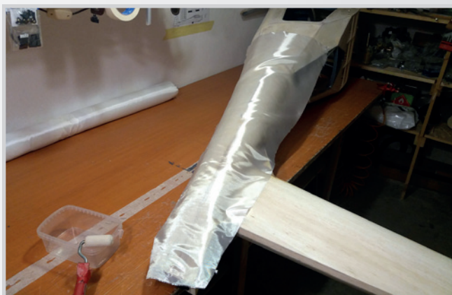
cover fuselage with fiberglass 50 g
