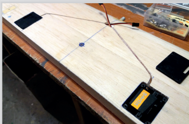
servo wires hide under balsa surface. it's better :-)
