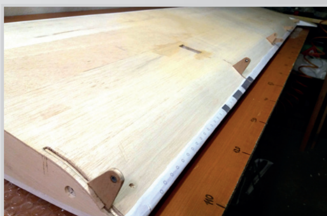
glued with PU
