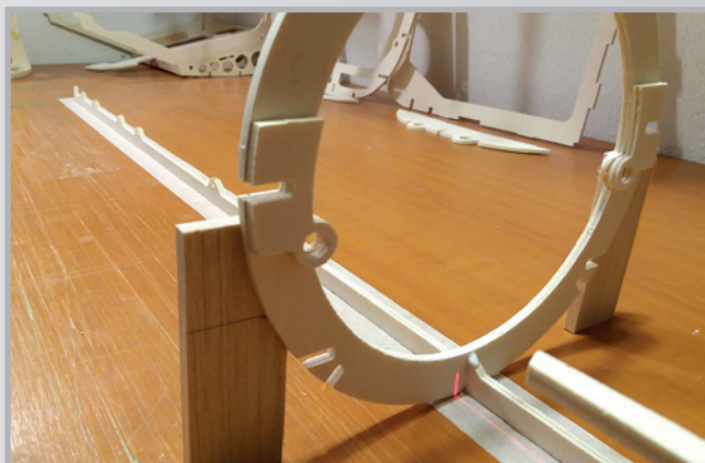
Use laser line to straighten all parts
