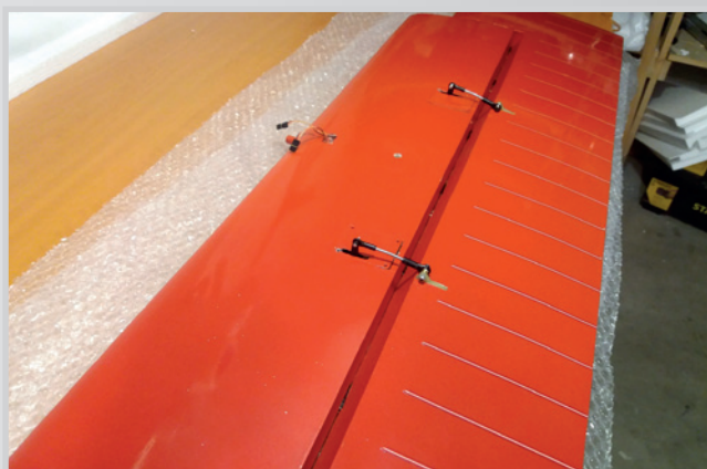
elevator servos installed
