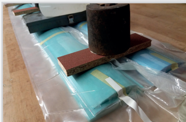
wing slats - 50 g fiberglass both sides in vacuum
