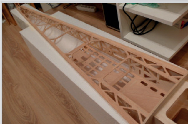
Gluing inside mold
