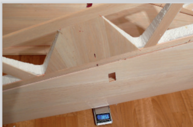
Aileron balsa cover: 1. possibility - cored (at photo) 2. possibility - whole aileron covered with one balsa sheet (simpler)
