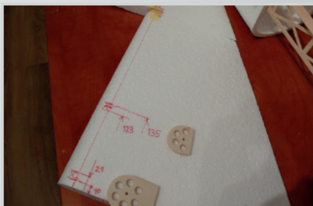
Half rib of rudder - bottom part is holding the rudderhorn
