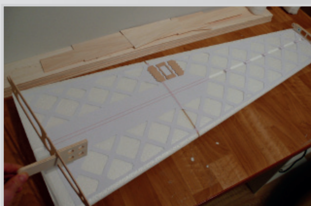
Preparations of two ribs and coring template
