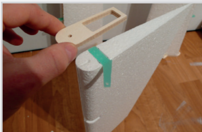
Cut little hole for elevator horn
