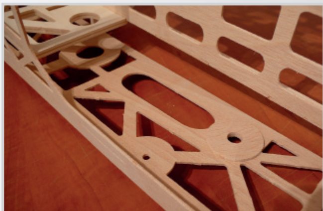
Inner reinforcements for wing tube casing and 10 mm pivots
