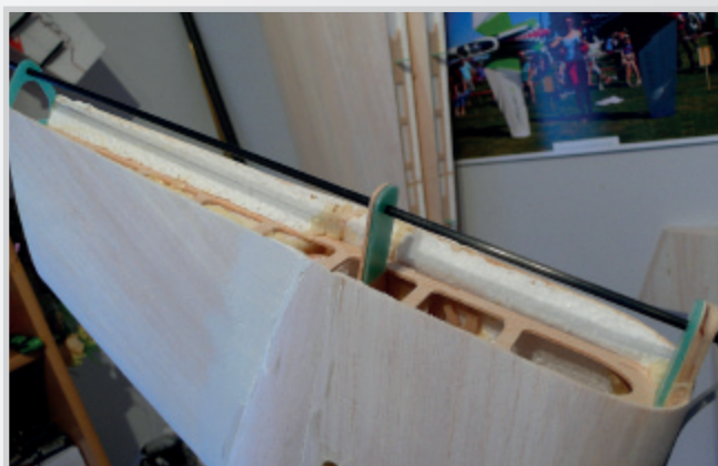
Fiberglass reinforcements of hinges
