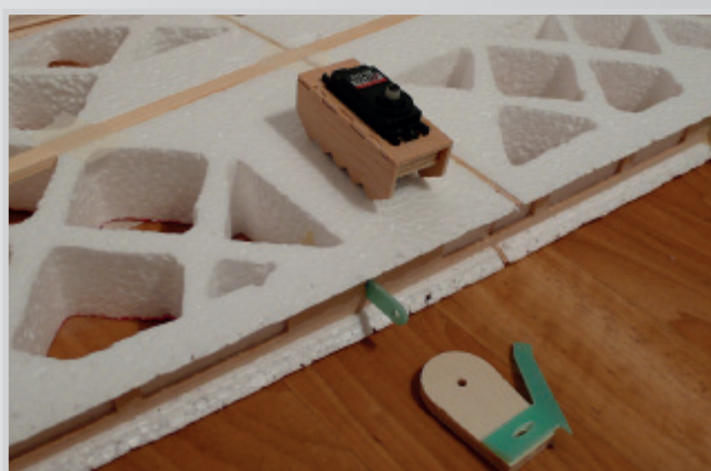
Servobox glued into wing core
