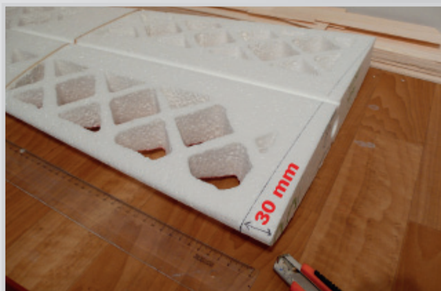
Cut the right angle and fit with fuselage
