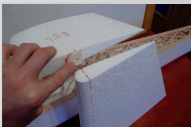
Half ribs of rudder
