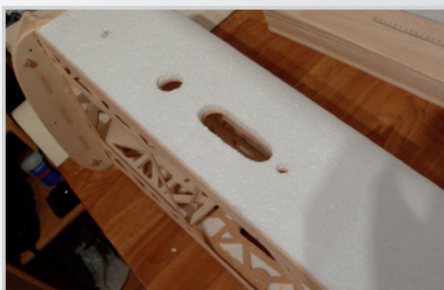
Holes for wing tube and pivots
