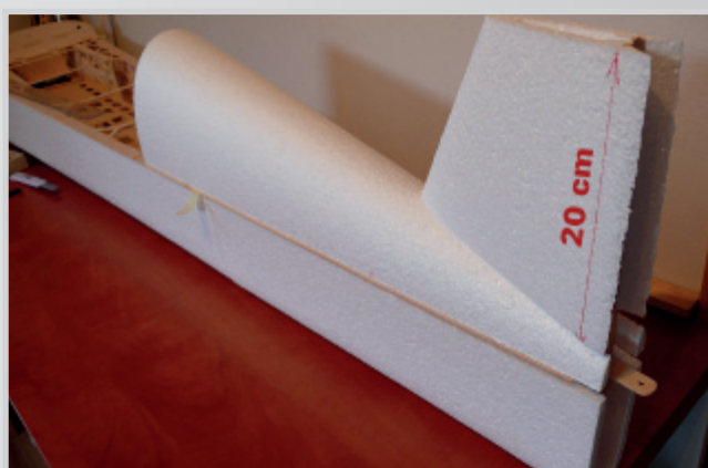
Cutting the right angle and lenght of rudder base
