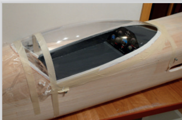
Finished cockpit glued with canopy
