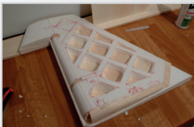
Covering with balsa 1,5 mm - use polyuretane glue
