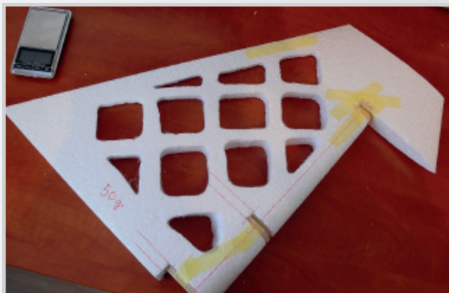
Coring of rudder base
