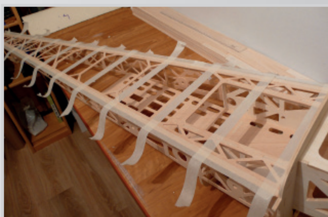
Preparation for gluing fuse construction with PS bottom part
