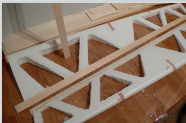
Aileron balsa cover: 1. possibility - cored (at photo) 2. possibility - whole aileron covered with one balsa sheet (simpler)
