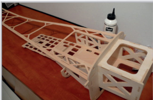
Gluing inner construction with engine lodge
