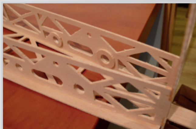
Reinforcements for elevator pivots and tube casing
