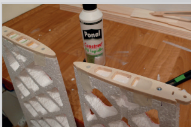
Nuts for SFG glued inside ribs
