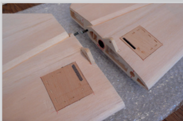
Servobox cover - glued just at finish after film covering of elevator (one of possibilities)
