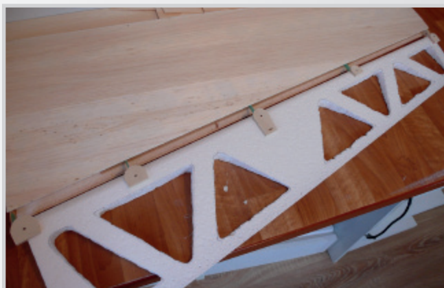
Gluing half ribs into aileron core
