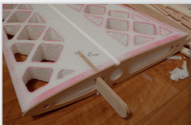
Gluing the rib and join wings part
