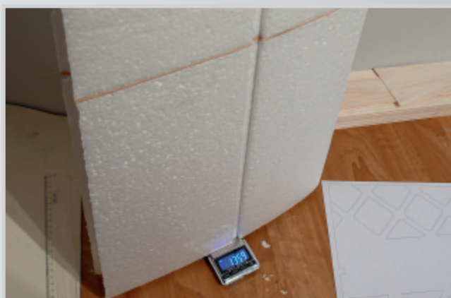
Gluing both parts of wing
