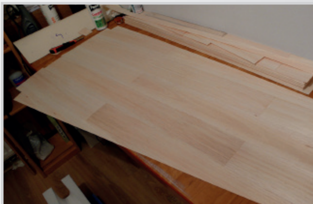
Preparation of whole balsa sheets for bottom fuse
