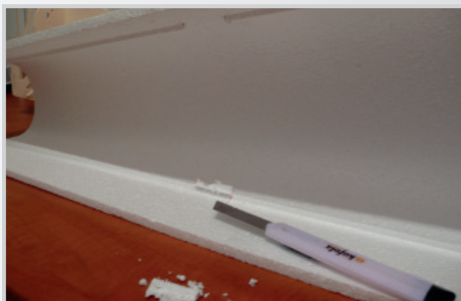
Cut little parts in the place of joining fuse base with bottom ply part
