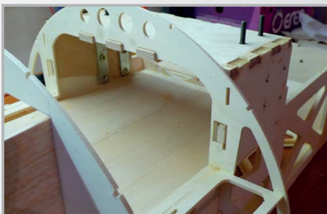
9. Gluing the undercarriage plate
