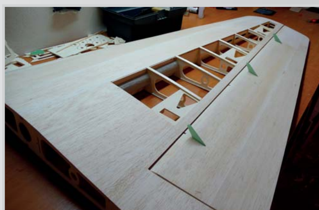
66. Cutting holes for levers - 2 or 3 servos can be used
