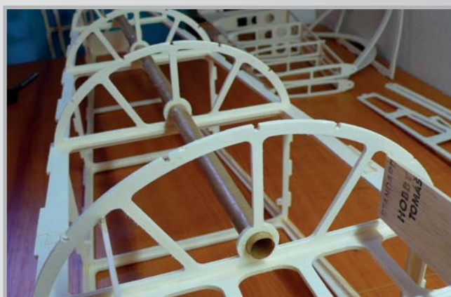
10. Paper tube for servo cables
