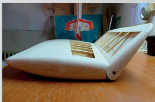
64. Cutting out the balsa overlap of the wing outlet - adjusting the sash deflection Cutting out the balsa overlap of the wing outflow - setting of the sash deflection
