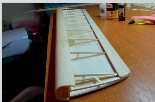
60. Secure with CA glue (or pins) on the edge of the main wing carrier
