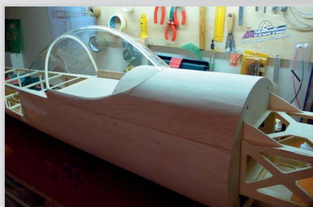
28. Coated top cover. Coated top cover with cab
