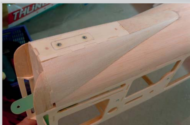
22. Balsa cover around spur dump
