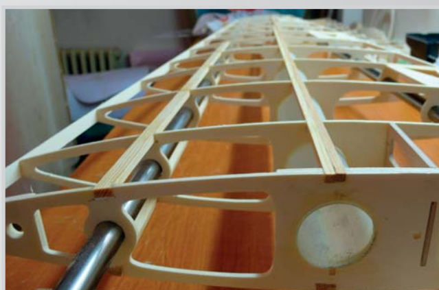
46. Double bar 5x5 over the depth upright and front bar 10x5
