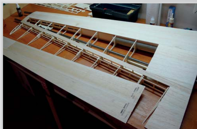
54. Preparation of the bottom side sheeting-B2
