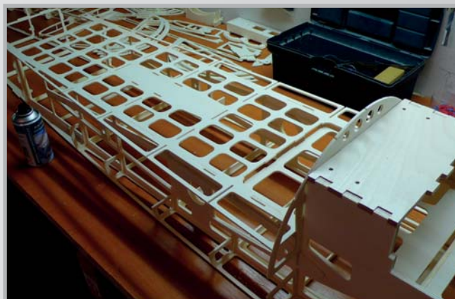
6. The chassis is not yet glued, the bottom plate in the fuselage yes
