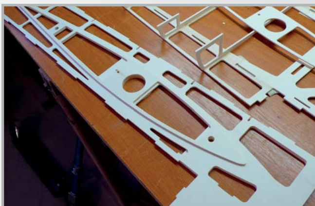
3. On the outside, the rib is glued (auxiliary for fitting the inner covering for flushing the wing)
