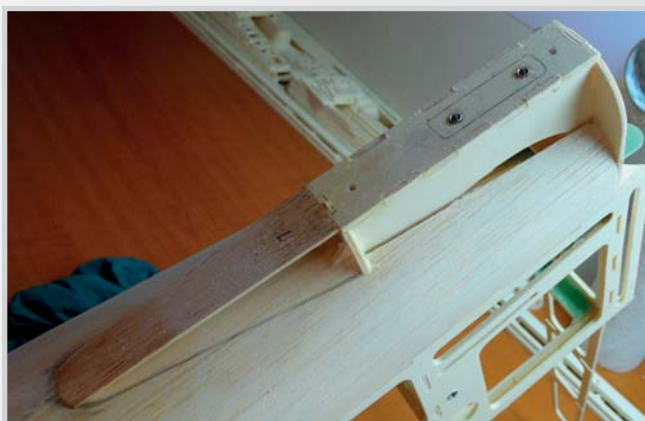
21. Spurge attachment (inside recessing nut M4)
