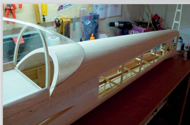
30. Turtledeck (sandwich polystyrene and balsa) glued to the hull with purex
