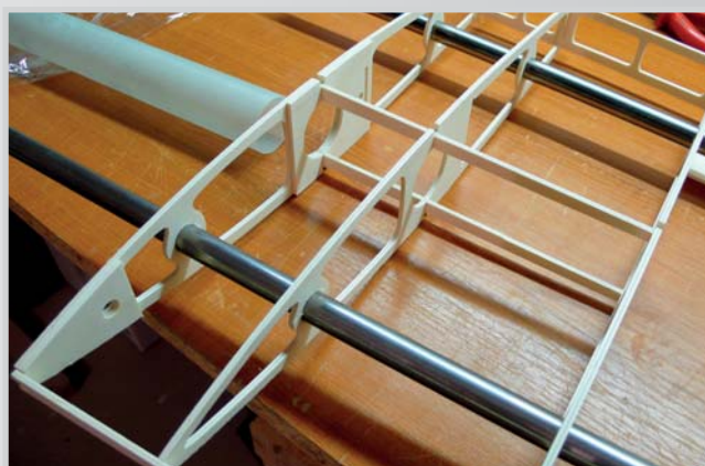
44. Rib ribs and auxiliary strips fitted
