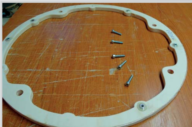
68. M4 nuts are sealed into the motor cover
