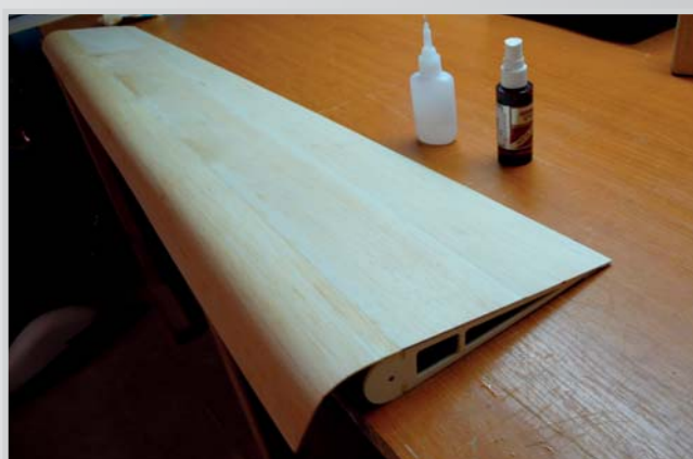
58. CA gluing with one edge adhesive
