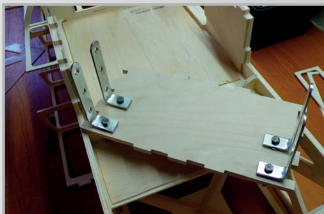
8. Preparation for attaching the undercarriage plate to the side fuselage
