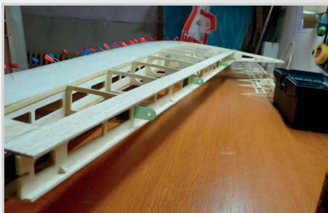
53. Hinges need to be sharpened slightly for slanting with the sash above and below
