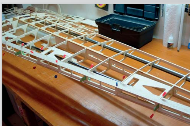
48. Gluing drainage bands - harder balsa 2mm (approx. 25mm wide)
