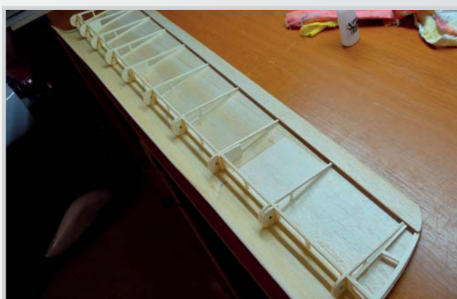
59. The rib faces are dispersed and the soft balsa is "wrapped" by pushing the wings against the table top
