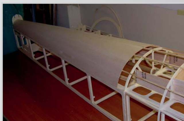
16. Beginning of b2 hull covering
