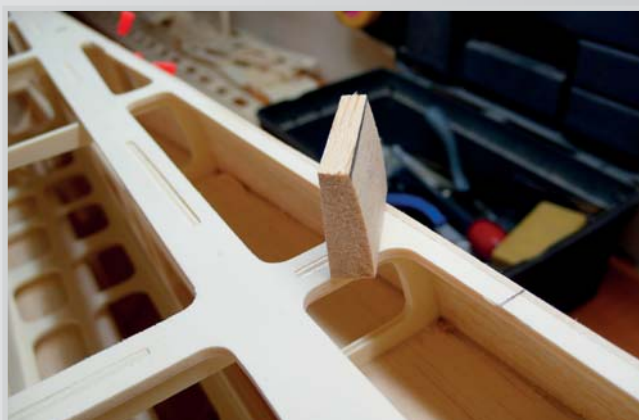
24. Preparing spacer blocks - holding the cab cover
