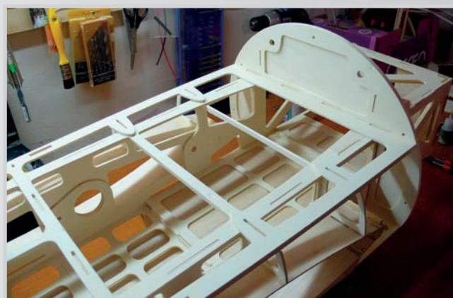
14. Glue the end of the hull that will hold the engine cover
