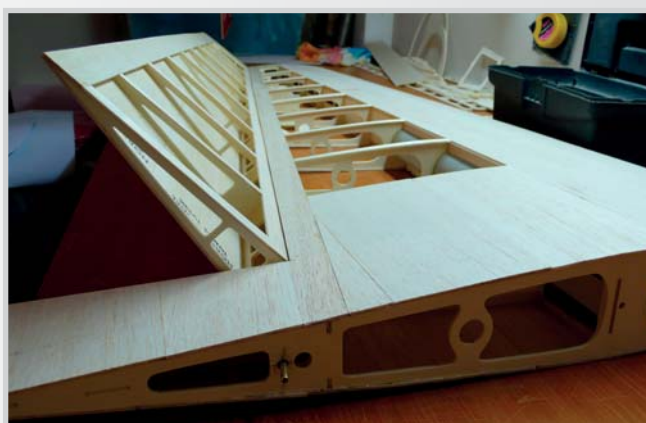
63. Incorporation of balsa overlap of the wing outlet - adjustment of the wing deflection
