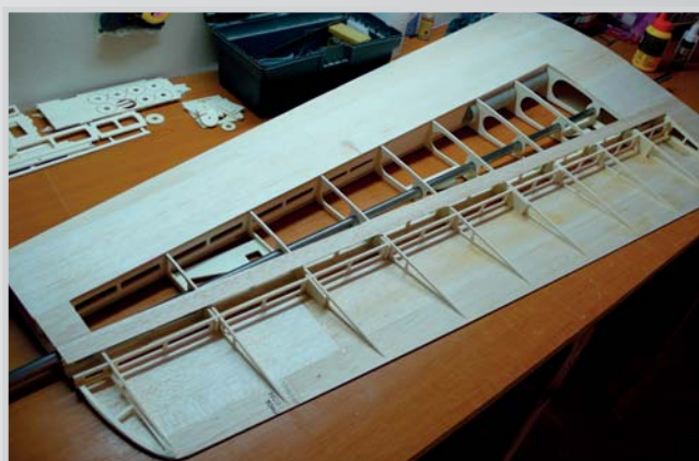
56. The drain strip is glued from the top
