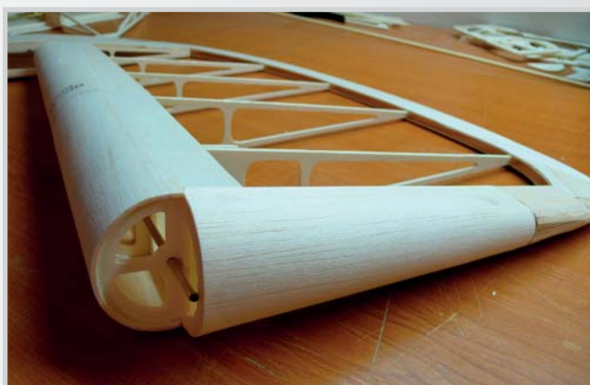
33. Bottom covered in the same way as the leading edge, only a thin end is glued a block of balsa
