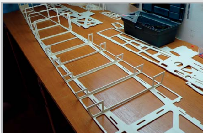
1. The construction of the hull begins "upside down"
