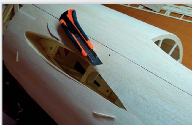
29. Cut out the wing opening
