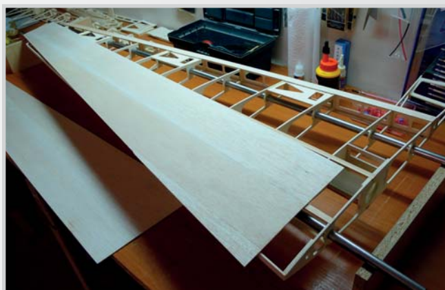
49. Ready and sanded sheeting of wing leading section
