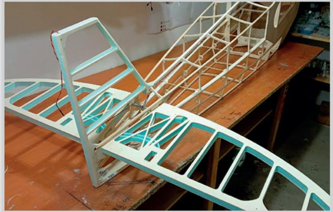
elevator with tubes 10 mm fitted to fuselage
