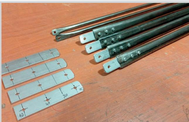
screwed and under screws filled with epoxy with microballoons
