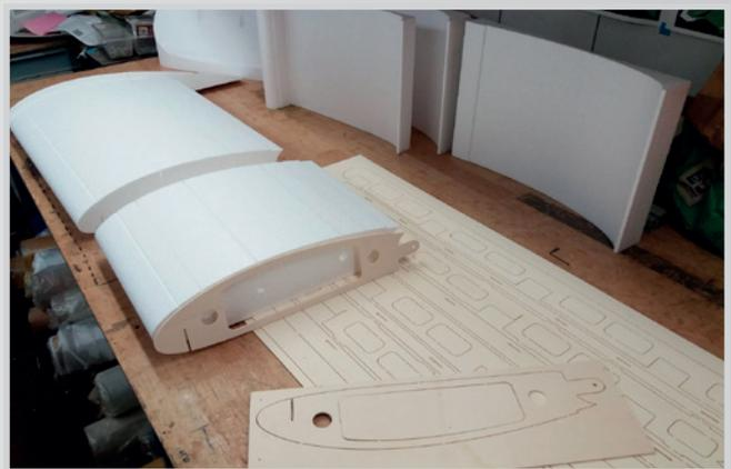
longest PS part (lef on the picture) you must cut into ribs 50 mm
