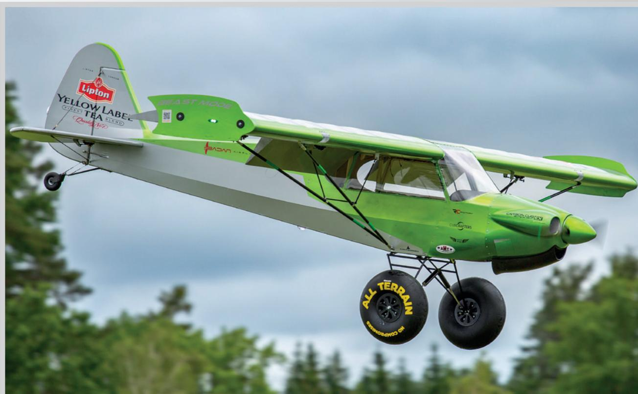
wingspan: 4,3 (4,7) m • length: 3,2 m • engine: 120-200 cc • weight: 18-22 kg
