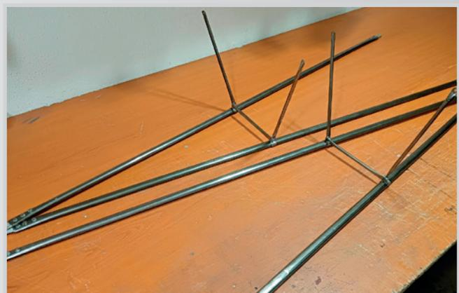
wing struts - thin wall steel tube. lenght about 1,4 m - NOT included in the kit - use thinwall steel or carbon fiber tubes about 15 mm
