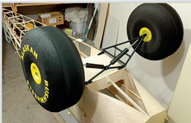
installed AMT landing gear
