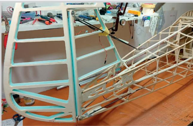
struts around rudder and elevator fitted to fuselage - NOT included in the kit
