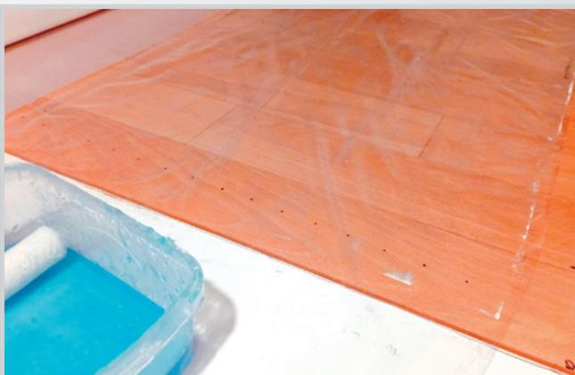
50 g fiberglass on thin plastic wrap - cut 3-4 cm stripes
