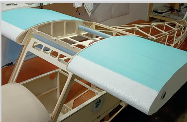
first wing parts on two 25 mm tubes - tubes 25mm with casings are included in the kit
