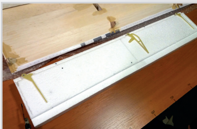
flap core with hinges - then cover flap with light balsa 1,5 mm
