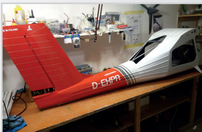
stripes stickers put on rudder and elevator before clearcoat
