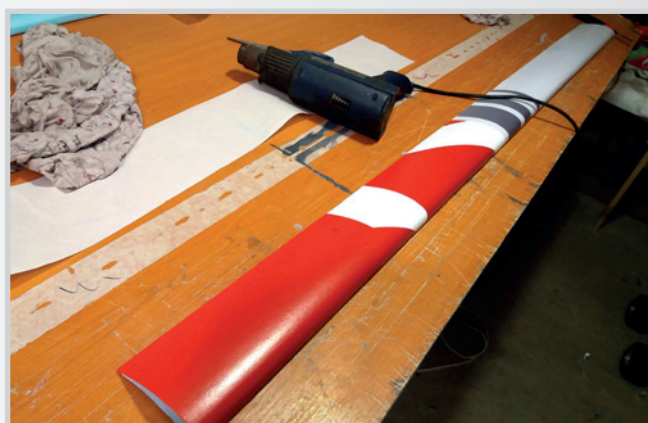
covering film applied directly on fiberglass surface. then it will be just clearcoated
