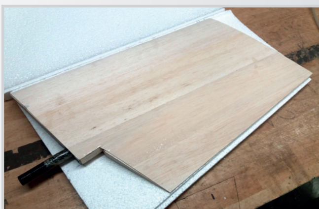
cover rudder with light balsa 1,5 mm
